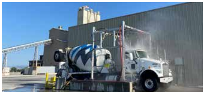
A recently added Shumaker Load & Go wash system reduces by at least 50 percent the normal truck wash down cycle and water consumption volume. All Load & Go water is captured in a nearby pit and pumped back to the weir system for reuse.
