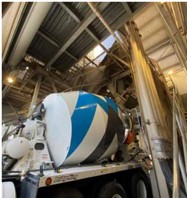
One employee-suggested plant feature is an internal watering system at loadout. It cools the drum during summer months and provides additional point source dust control during truck charging.
